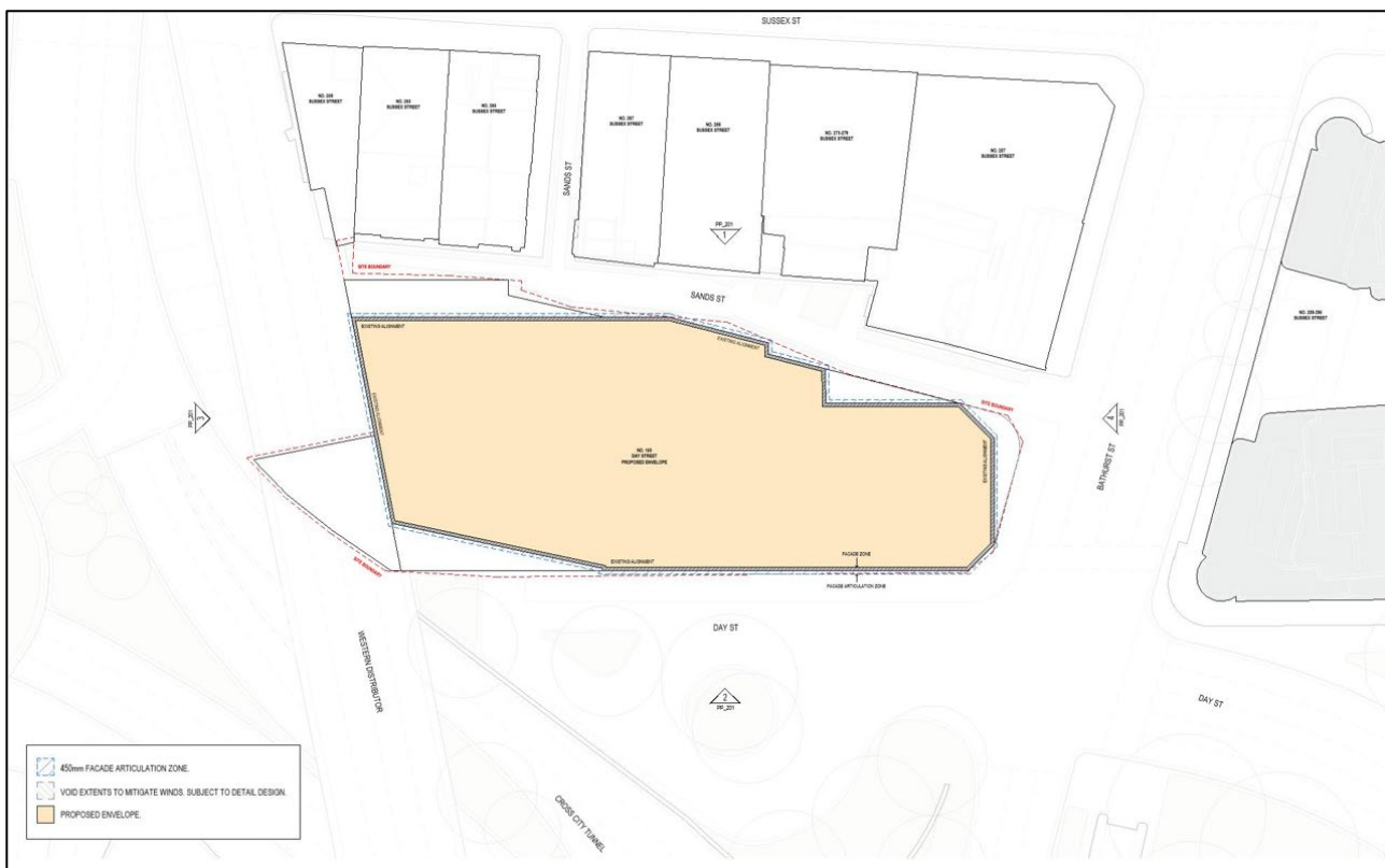
Figure 19 Building Envelope – New Tower Setback (Level 13-17 Floor Plan) Source: Hassell
