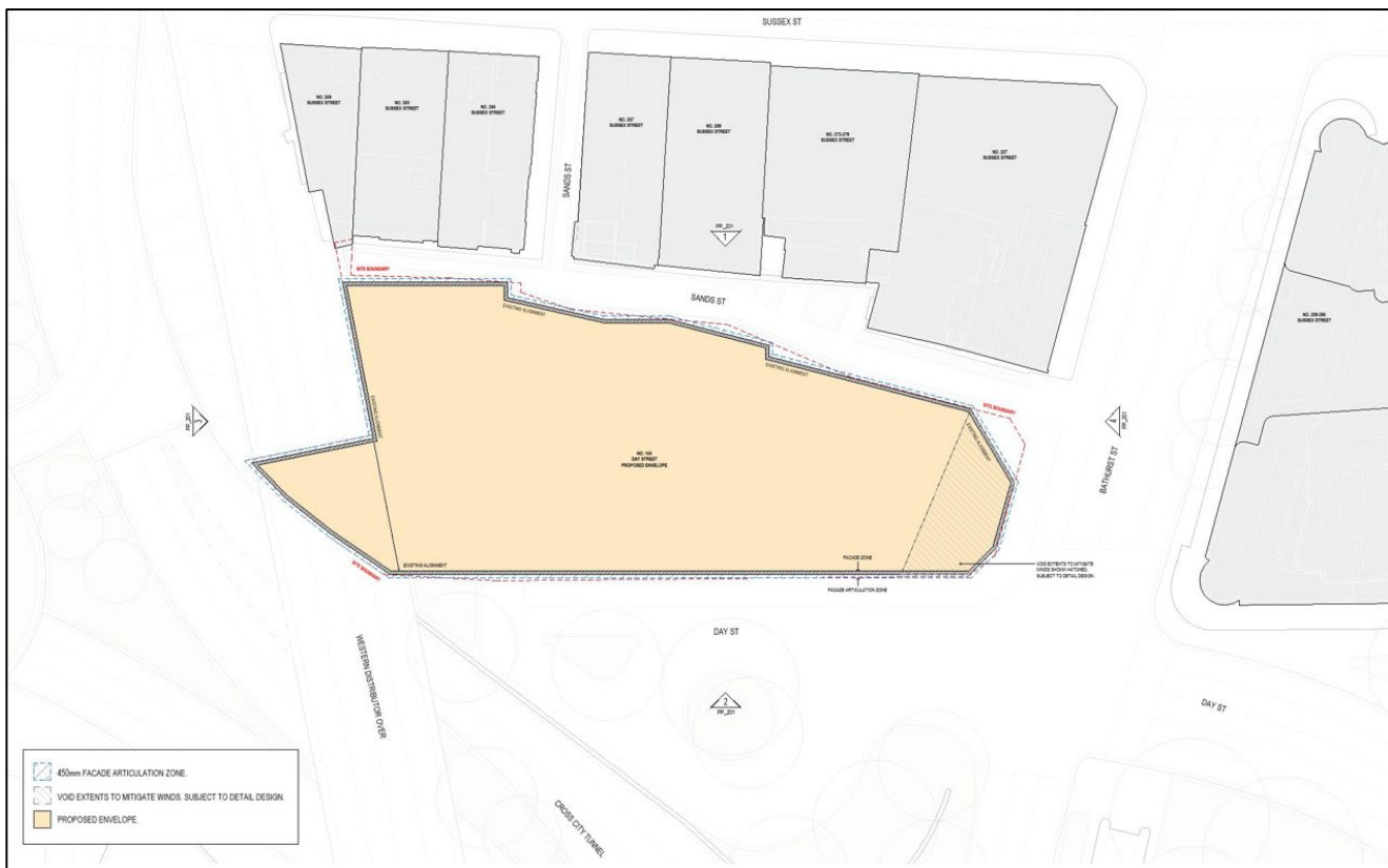
Figure 17 Building Envelope – Podium Setback (Ground Floor Plan) Source: Hassell
